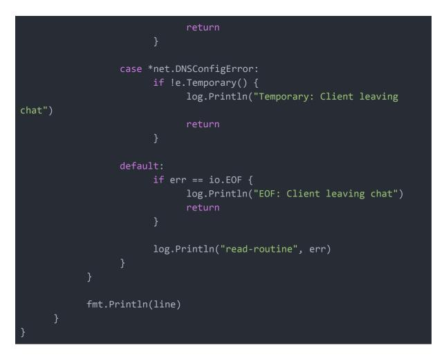
temporary is declared to test for the existence of the method coming from the net package. Because Temporary is the only behavior we care about. If the concrete type has the method named temporary then this is what we want. We get to stay decoupled and continue to work at the interface level.
