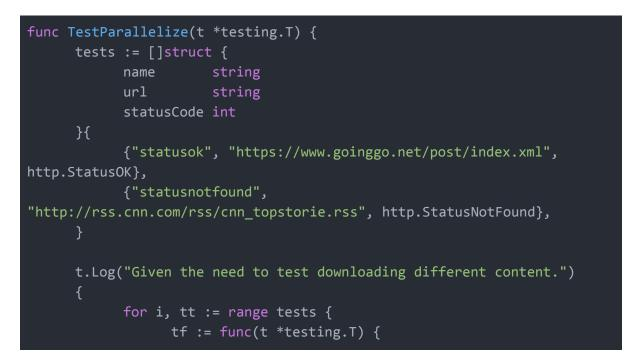
The only difference here is that we call Parallel function inside each of these individual sub test functions.
