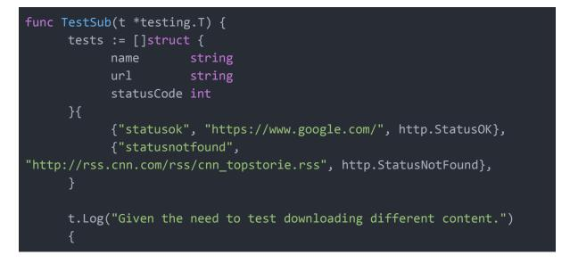
Range over our table but this time, create an anonymous function that takes a testing T parameter. This is a test function inside a test function. What's nice about it is that we are gonna have a new function for each set of data that we have in our table. Therefore, we will end up with 2 different functions here.
